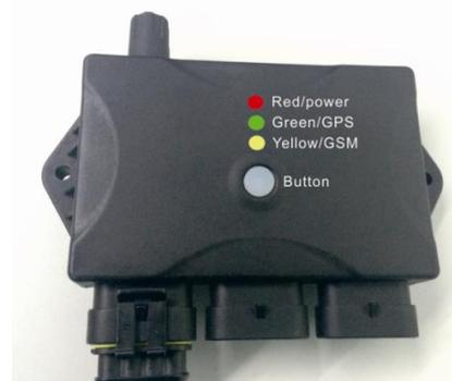
The module receives tyre pressure and temperature data from sensors on the tyres and location information from the GPS. This data is transmitted through the network connection every few minutes. In the event of an alert condition, the normal transmission sequence is interrupted and data is transmitted immediately.
